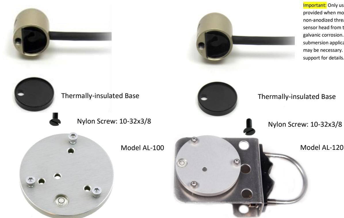
To minimize azimuth error, the sensor should be mounted with the cable pointing toward true north in the northern hemisphere or true south in the southern hemisphere. Azimuth error is typically less than 1 %, but it is easy to minimize by proper cable orientation.
